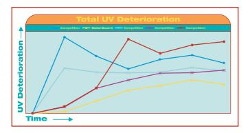
SolarGuard<sup>™</sup> maintained stability in thickness proving that its physical properties remain very much intact despite EMMAQUA testing that concentrates natural sunlight using 10 highly reflective mirrors to create an intensity level of approximately 8 suns!
